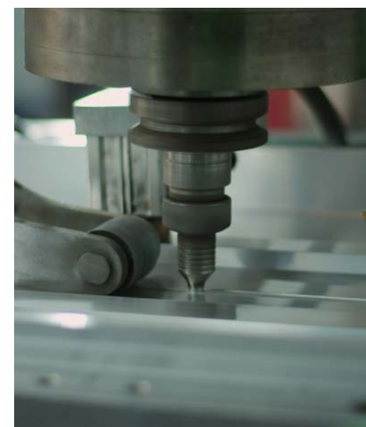
FRICTION STIR WELDING (FSW) / 搅拌摩擦焊
